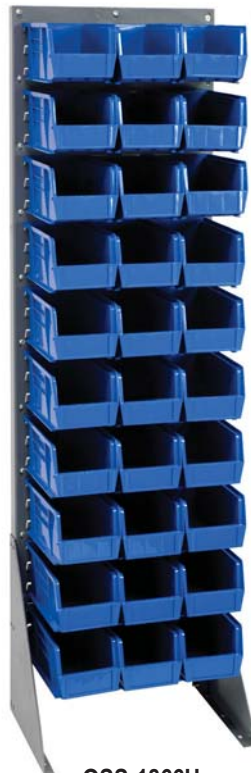
QSS-1866H Single Sided Louvered Rack 18"L x 12-1/2"W x 66"H Single sided unit accepts all sizes of Ultra Bins (up to 60 bins) 375 lb. capacity. (Bins sold separately)
